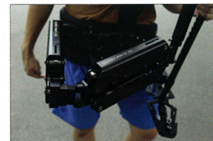
The support arms of the X-10 can accommodate both left-handed and right-handed individuals.
