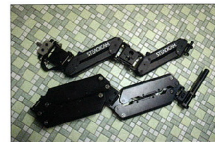
The support arms, as well as the rest of the setup, can be easily dismantled for convenient transport.
